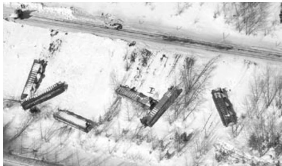
The aftermath of the January, 2004 avalanche cycle in John F. Stevens Canyon where slides struck a train of empty grain cars. The derailed cars were pushed off the railbed in order to speed cleanup in hazardous conditions. *Photo by Darwon Stoneman*
