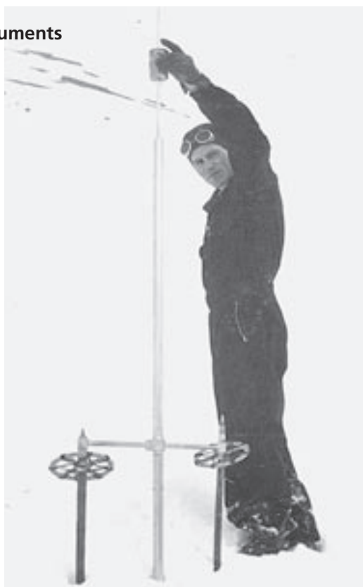
Cone penetrometer for measuring ram resistance.
