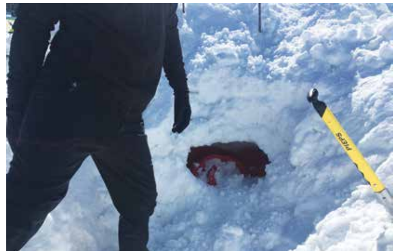
Figure 2. Example of the air pocket created by deflation of the airbag observed upon extrication.
