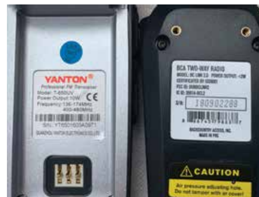
The radio on the left has no FCC Identification number—and is therefore illegal to operate or sell. The radio on the right has an FCC ID number, which means it complies with Part 90 of the FCC regulations.
